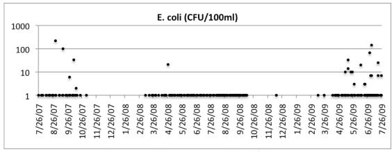
Figure I-2: Control chart of E. coli blanks
